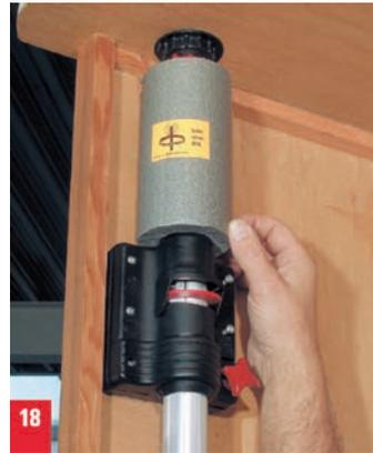
18. Put an insulating sleeve between the mounting bracket and the ceiling (not included in the scope of delivery, recommended for winter caravanning).
