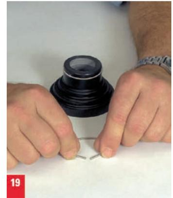
19. If it is necessary to retighten the circular spring, shorten it by nipping off ca. 2 mm.
