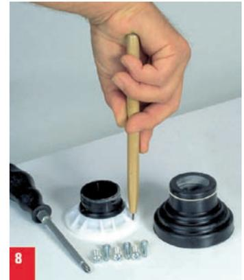
8. Use a gimlet to make holes in the roof duct. If your vehicle has a plastic roof, pre-drill holes using a  $\varnothing$  3.5 mm drill bit.
